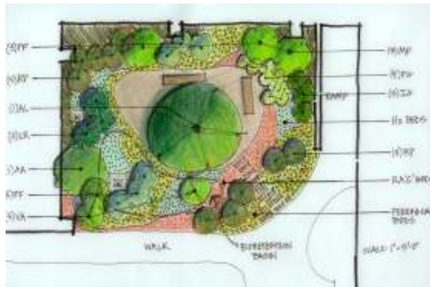
Figure 2: Concept Design for Rain Garden eligible for inclusion in required open space
